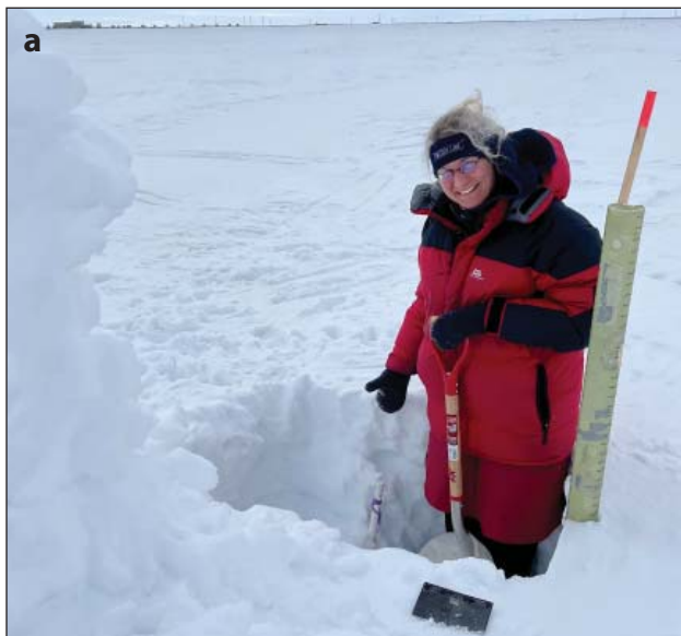
Figure 11. Snow character at a relatively dust-free site and a site with heavy road dust. a. Anja Kade and snow pit at the relatively dust-free NIRPO site in a thermokarst pond with deep snow. Note the top of the 120-cm snow stake, which is anchored in the bottom of the pond; at least half of the stake is below the water level in the pond. b. Olivia Hobgood and snow pit at a dusty polygon-center plot along the Spine Road at the Colleen site. Note the ESC30 snow sampling tube in both photos. Both photos were taken 2 May 2022. (Credits: A.L. Breen, IMG 0192, IMG 0182)
