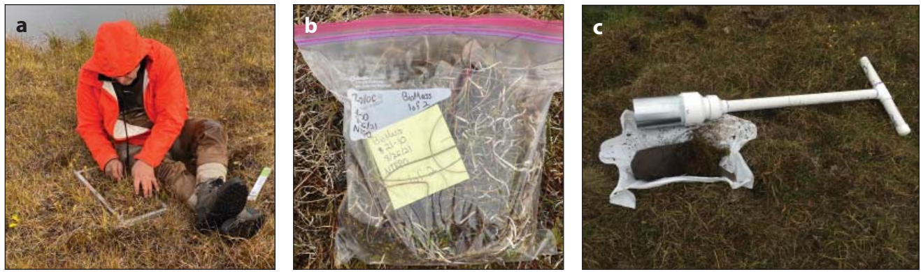
Figure 6. Biomass harvest methods. a. Cutting out a 50-cm x 20-cm slice of tundra using a metal frame and a bread knife. b. Ziploc® bag containing one half of the tundra slice. c. Coring device used to sample biomass and soils in aquatic sites. (Credits: J.L. Peirce, IMG 5608, IMG 5602; E. Watson-Cook, IMG 3631)
