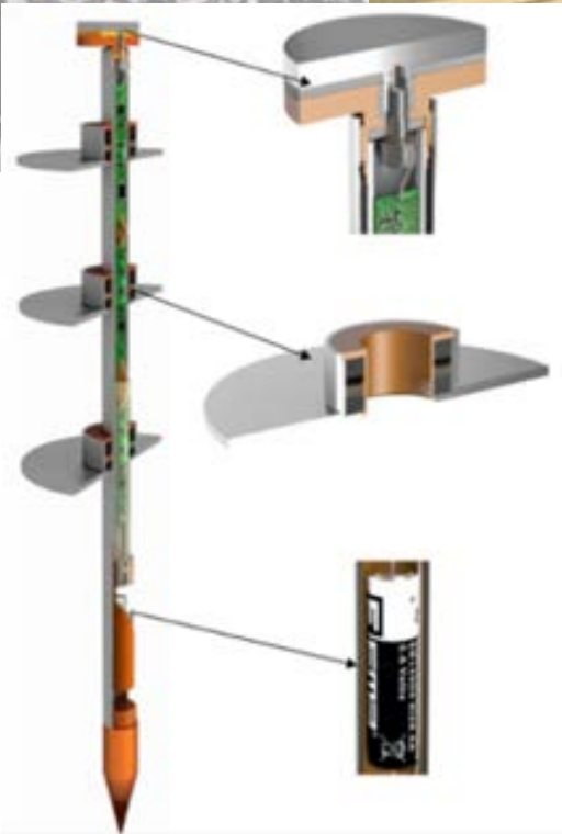
Location of pressure, deformation and humidity sensors in the road structure.
